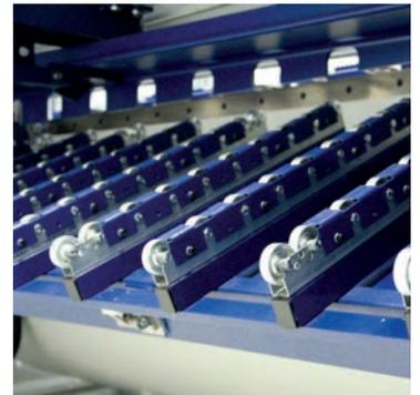
Sheet support, pneumatically controlled
