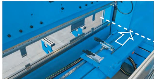
Relative X1-axis for gauging of e.g. conic parts.
