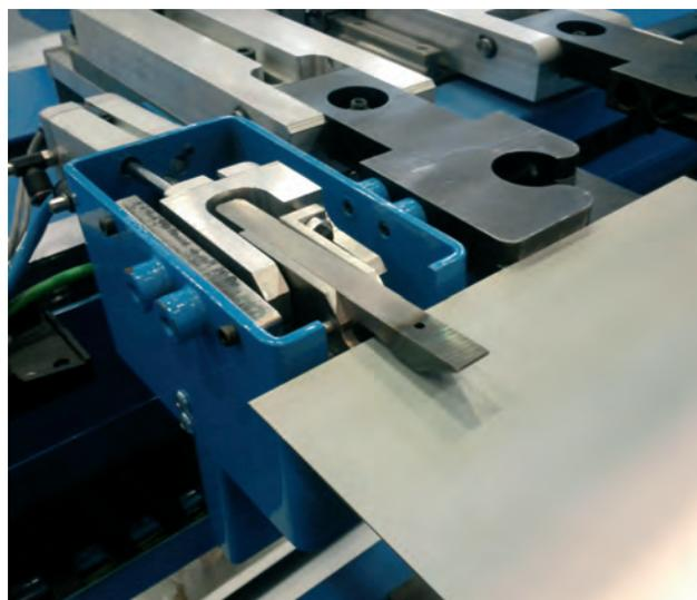
The Prima Power **TMS** Thickness Measurement System provides reliable and fast thickness measurement. The TMS is mounted next to the left back gauge finger allowing thickness measurement simultaneously with part gauging. Thanks to the integration into the Prima Electro Open Control measuring results are automatically transferred to NC program without operator intervention.
